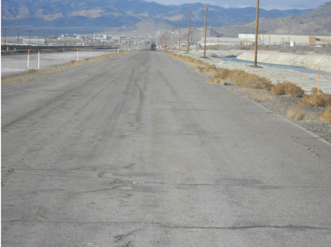
Front Tire Marks at Maximum Effectiveness; Toyota Camry – All Brakes Working.
