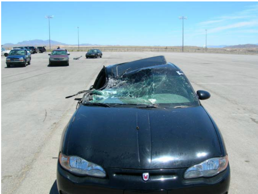
Figure 2. Frontal view of roof damage of Monte Carlo.
