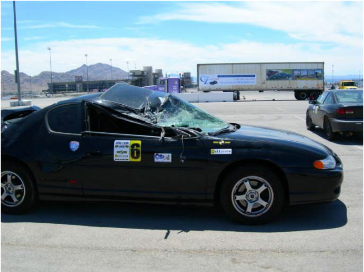
Figure 3. Side view of Monte Carlo roof damage.
